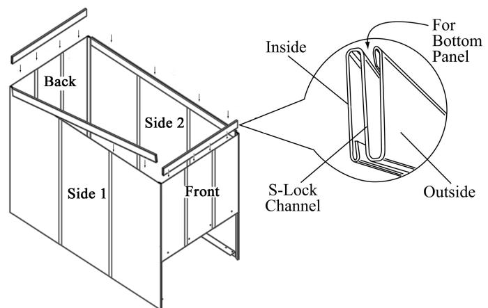
Step 5. Place the box upside down and slide the short S-Locks onto the bottom edges of the Front and Back panels and the long S-Locks onto the bottom edges of the Side panels while ensuring the open S-Lock Channels are on the outside of each panel as shown.
