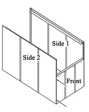
Step 2. Snap Front panel into the end of Side panel 2 with furnace support facing up as shown.
