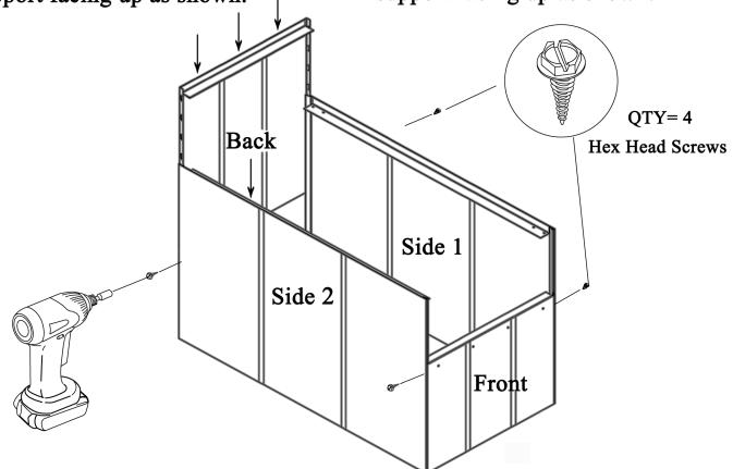
Step 3. Snap Back panel into the ends of Side panel 1 and 2 with the furnace support facing up and slide down as shown. <u>Step 4.</u> Ensure the bottom edges are even and all sides are aligned then drill(4) hex head screws into the Side panels at the locations indicated.
