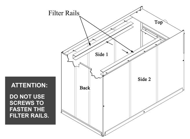
Step 9. Slide the (2) Filter Rails onto the filter box furnace supports on the Side panels and then slide them all the way back so they are secured between the furnace supports on the Back panel and Side panels.
