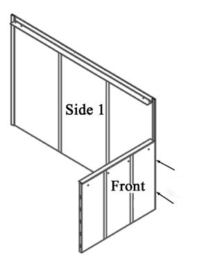
Step 1. Snap Front panel into the end of Side panel 1 with furnace support facing up as shown.
